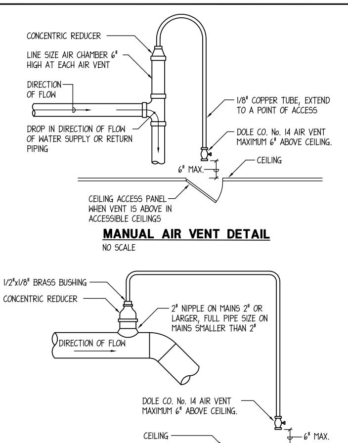
AIR VENT AT HIGH POINTS OF MAINS NO SCALE
